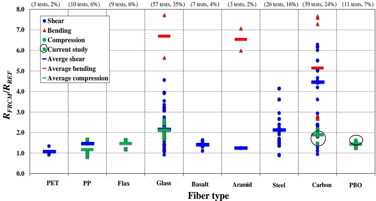
Figure 6 - Distribution of  $R_{FRM}/R_{REF}$  as a function of fiber type
