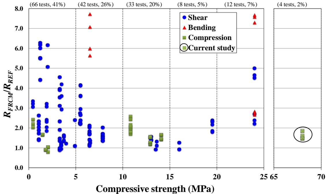
**Figure 5** - Distribution of  $R_{FRM}/R_{REF}$  as a function of concrete and masonry compressive strength
